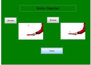
According to these images we detect the motion and optical flow. Here using the optical tool box and computer vision toolbox. For motion detection Ransac algorithm is used here and Lucas Kanade algorithm for optical flow. In Ransac first feature is detect then extract the feature and then find out the matching points and find out the motion is happened or not. Then plot optical flow, for this lines are using here and show the movement of pixels. Here display the possible movement of pixels.
